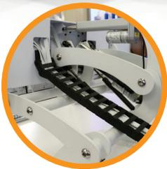
Cables are routed through an E-chain cable management system for clean and efficient routing and bundling.
